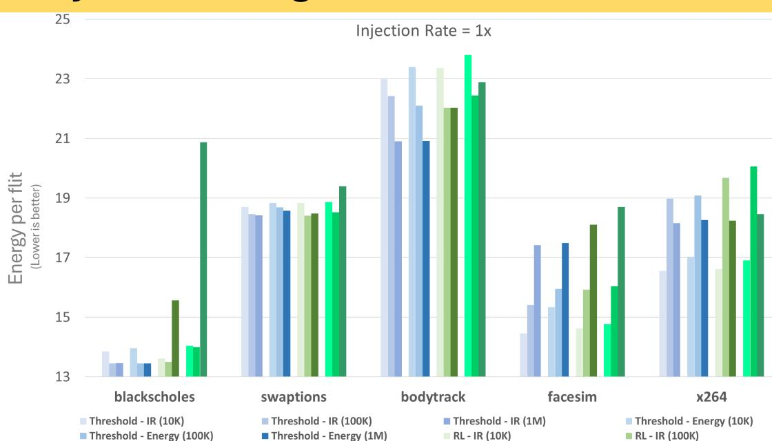
The *Energy per flit* includes the energy for flit transport AND switching the topology.
